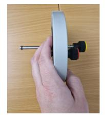
Reassemble the hook on the rod of the 5555-10-TC
