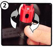
Tighten the connector Hub firmly onto the JOOLTOOL spindle.
