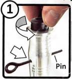
Insert pin into Handpiece. Unscrew & remove the collet nut. Note: Collet size must Use wrench if needed. match shaft size of bit.
