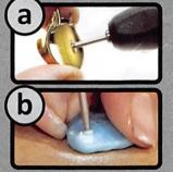
a) Use small brushes for intricate sanding and polishing in hard-to-reach areas.(b) Use Diamond & Drilling bits on a variety of materials, even stones!
