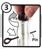
Insert & screw collet nut. Do NOT tighten yet.
