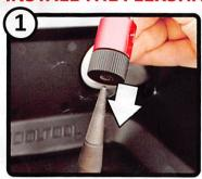
Slide the Flexshaft Connector Hub onto the Jooltool spindle. This is similar to installing Backpads onto the Spindle.
