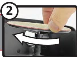
Twist the disc onto the Spindle until locked, but do NOT overtighten.
