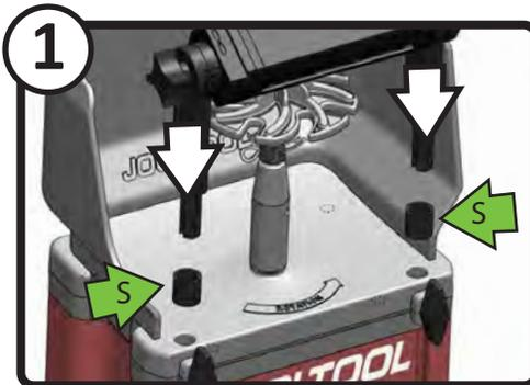
Slide the Posts into the mounting holes as shown. **Locking knob will be on left-hand side when properly mounted.**
