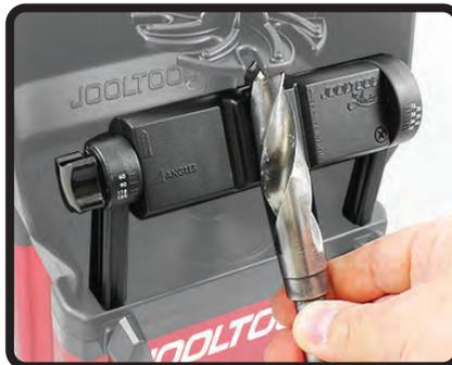
Use the Tool Rest to get sharp and precise angles on chisels & drill bits. (see "TOOL REST CHISEL SIDE" & "TOOL REST DRILL BIT SIDE" in this guide)
