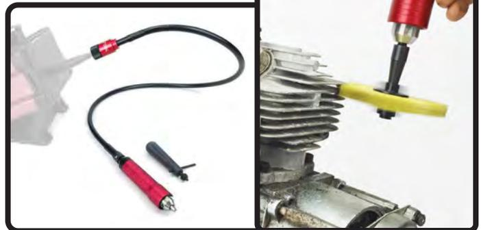
The Flexshaft attaches to heavy-duty Handpieces to use Dremel-type bits, Drilling burs, power carvers, sanders and more... (see "Jooltool HD FLEXSHAFT" in this guide)
