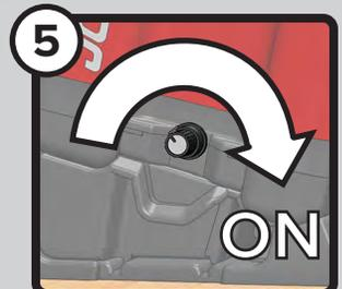
Turn the speed control knob **clockwise** to turn the machine ON and test at various speeds. RESET IS COMPLETE!
