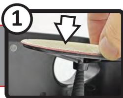
With abrasive side UP, slide the disc onto the spindle of your JOOLTOOL.
