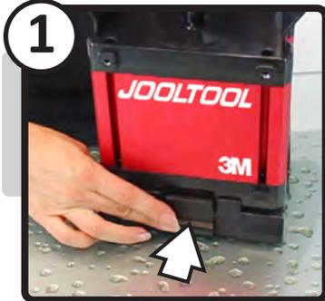
1 Press EJECT BUTTON to release the tool from base.
