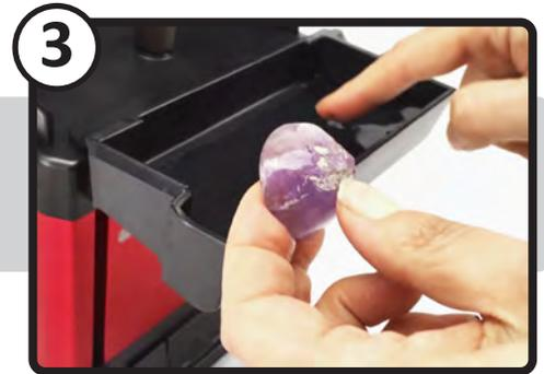
3 The drawer/water tray can hold water for quick access to lubrication when performing lapidary work.
