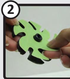
Align See-Thru design with Backpad slots and press firmly to adhere.
