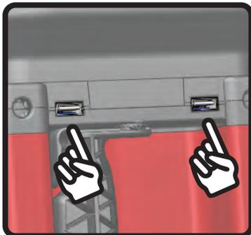
The 2 convenient rear USB ports can power LED lights or charge your mobile devices. **Anie recommends to keep your machine stationary while charging.**
