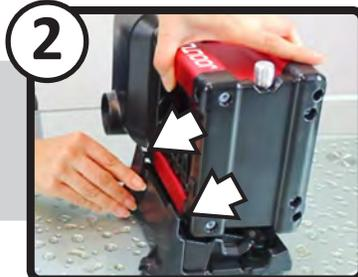
2 Set the Jooltool to its side and align the Holes at the rear of the Tool with the ALIGNMENT PINS on the BASE. Speed control switch will be pointing upward when properly docked.
