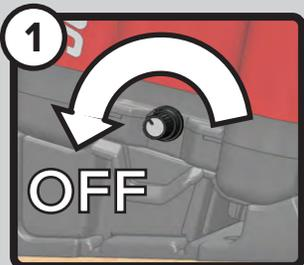
Turn the speed control knob **counterclockwise** to turn the machine OFF until you hear a "click".
