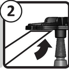
**STEP 2:** Touch the entire width of the edge flat against the disc. Hold in place.
