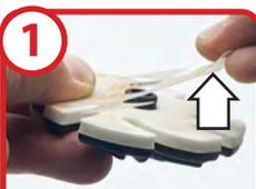
Remove the worn abrasive (top film)
