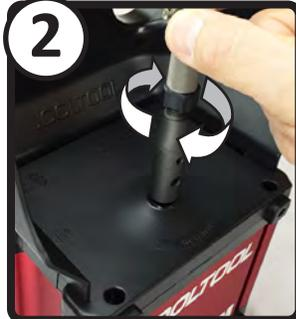
**(2.1)** Twist clockwise onto the Spindle of the JOOLTOOL using grip areas at the bottom of the mandrel.
