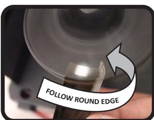
For workpieces with rounded edges, keep in mind that they generally have a **FLAT** EDGE which simply contours the rounded surface of the workpiece.
