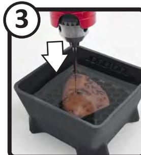
Anie's STONE & PEARL DRILLING RESERVOIR keeps pieces lubricated as your drill in water.
