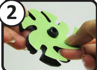
**ALWAYS** place abrasive on the FLAT (BOTTOM) surface of the BACKPAD.
