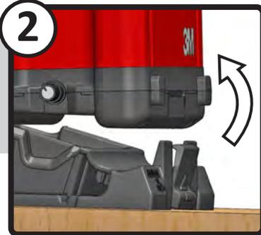
2 GENTLY tilt machine upwards
