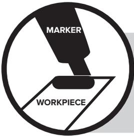
**ANIE'S TIP:** To improve visibility of the surface or edge you are working on, darken it with a black marker (Sharpie™) or use a marker color that contrasts with the surface to be worked. The marker gets erased on contact with the abrasive.
