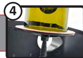
Turn the machine ON and work on the TOP ABRASIVE to shape & polish stones, bottles, etc.
