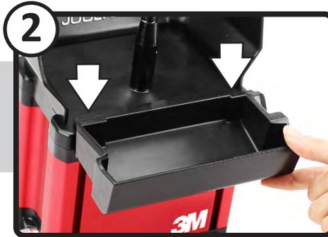
2 The drawer transforms into a handy water tray. Slide it completely off the tool, then mount it by inserting the 2 locator pins into the 2 holes at the top of the Jooltool.
