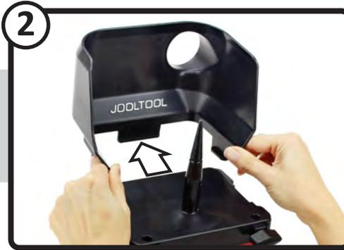
2 Slide the Hood out and away from the Jooltool. Reverse steps 1 & 2 to reinstall (Center the rear tab, pull towards you, snap tabs back into their slots)
