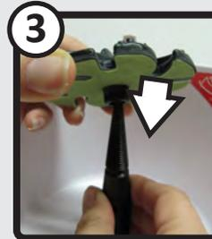
With abrasive side DOWN, place the disc onto your Jooltool Spindle.
