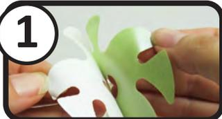
Remove all protective film from new ABRASIVE before applying it onto the BACKPAD.
