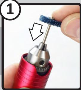
Insert the desired bit into the handpiece chuck/jaw. **Note:** Jaw must be opened wide enough to fit your bit.
