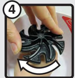
Twist the disc assembly onto your Jooltool Spindle. Twist until locked, but do NOT overtighten.
