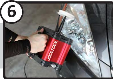
6 The Jooltool is also great for removing scratches from headlight lenses and gently buffing clear-coated surfaces using slow speed settings.
