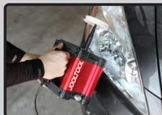
Use **JOOLTOOL'S** portable mode with the **FLUFFY COTTON BUFFING WHEEL** for removing scratches from headlight lenses or for buffing large items.
