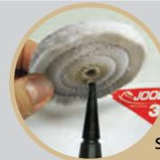
Twist onto the spindle to **INSTALL**
