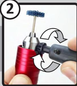
Using the chuck key, tighten the jaw. **Note:** Check if the bit is centered by rotating the chuck by hand.
