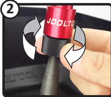
Tighten the connector Hub firmly onto the JOOFTOOL spindle.
