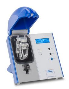
Watch leak detector for the professional use. Perfect for watches with or without watch strap. Leak detection through pressure and/or vacuum. Simple handling with 7 predefined universal testing programmes plus one special programme for locating the leaks. 10 additional testing programmes available, adjustable according to individual requirements.
