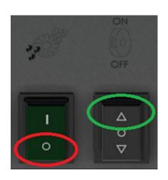
3. When Vacuum motors is off position push the polishing motor's on/of button several times and listen very carefully. Because during this operation, you should hear a special sound (a tick sound) which come from inside of the machine( it will come from contactor )
