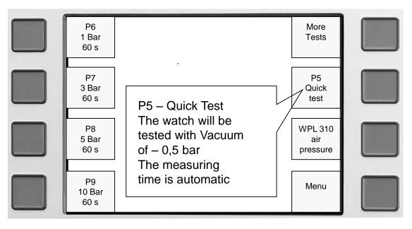
P6 = Pressure = 1,0 bar / Measuring time = 60 seconds P7 = Pressure = 3,0 bar / Measuring time = 60 seconds P8 = Pressure = 5,0 bar / Measuring time = 60 seconds P9 = Pressure = 10,0 bar / Measuring time = 60 seconds
