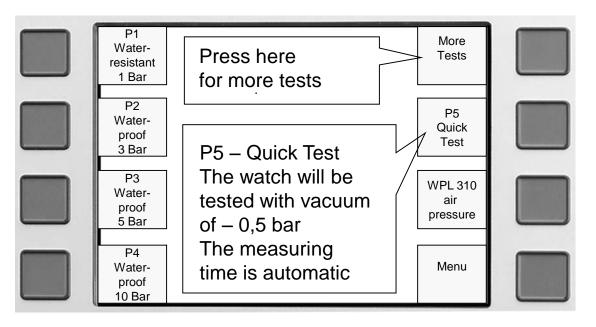
P1 = Vacuum - 0,5 bar / Pressure = 1,0 bar / Time = automatic. P2 = Vacuum - 0,7 bar / Pressure = 3,0 bar / Time = automatic. P3 = Vacuum - 0,7 bar / Pressure = 5,0 bar / Time = automatic. P4 = Vacuum - 0,7 bar / Pressure = 10,0 bar / Time = automatic.
