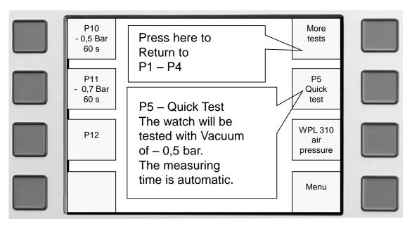
P10 = Vacuum - 0,5 bar / Measuring time = 60 secondsP11 = Vacuum - 0,7 bar / Measuring time = 60 secondsP12 = Not programmed
