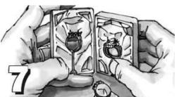
Parting lines are easily controlled and corrected by hand when used with the powder separation technique.
