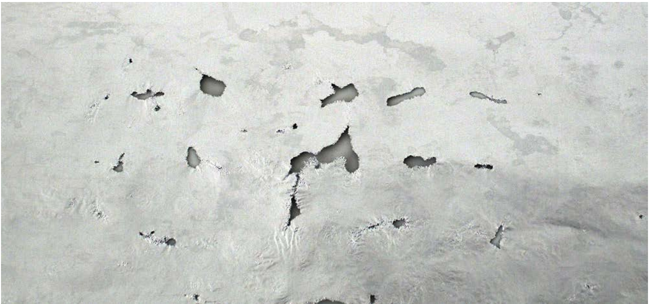
Example: aluminum foil after ultrasonic treatment in an Elmasonic S30.
