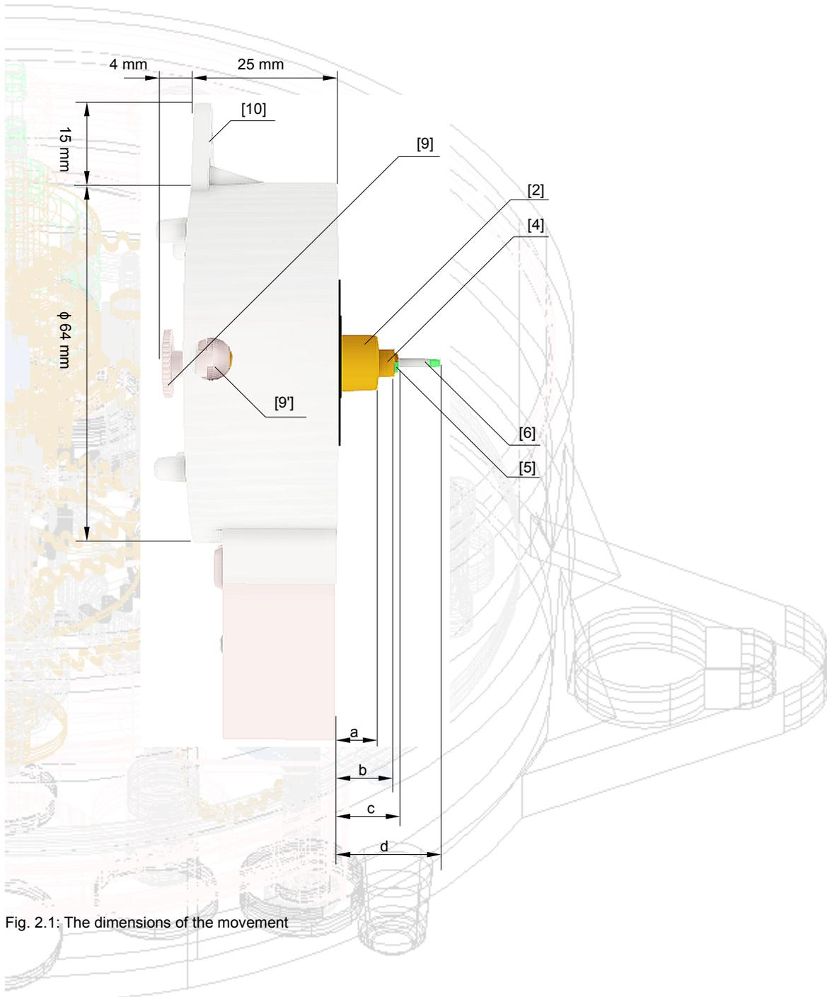
Fig. 2.1: The dimensions of the movement
