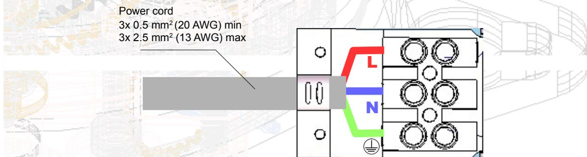
Fig. 3.3. Assembly of the power cord into the block connector [11]
