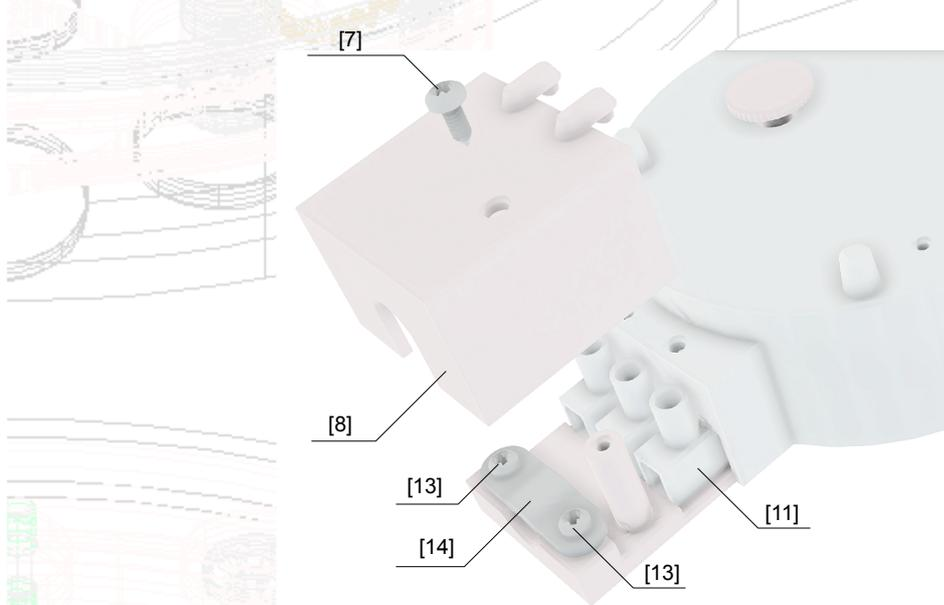
Fig. 3.2: Disassembly of the terminal cover
