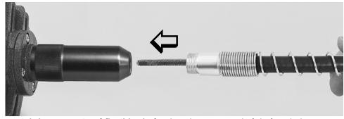
**3.** Lightly grease tip of flexible shaft. Align the square end of shaft with the square hole in the shaft adapter. Finally, screw the outer sheath into the motor connector.
