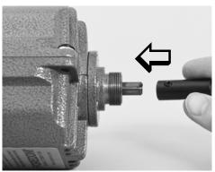
**1.** Place shaft adapter on motor hub. Align set screw with flat side of motor hub and tighten with hex key.
