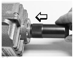
**2.** Screw motor connector onto motor. Motor connector has a left hand thread and must be turned counterclockwise (left) to tighten.
