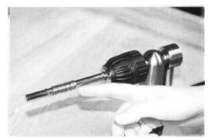
3) Cut the wire near the mandrel (A) and then cut the wire which is inserted in the hole (B). Now slide the coil off mandrel.
