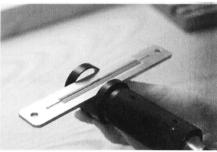
**10)** To double check, place lid of coil holder onto the flex shaft holder and ensure that the blade is in the middle of the groove.
