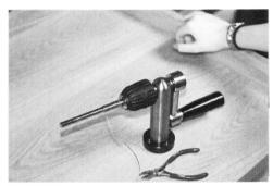
2) Insert the end of the selected wire into the hole of the mandrel. — (There are no holes on mandrel sizes 3mm, 3.5mm & 4mm). On these sizes, place the the wire between two of the chuck teeth. Hold wire firmly in your left hand and turn the coil winder (black handle) clockwise with your right hand. Hold the wire against the coil. — So having the wire always slightly to the right of the coil. This will ensure a tight coil. A tight coil is necessary to make good jump rings.
