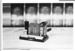
1) Select a mandrel that will be the inside diameter of your Jump Rings. Insert the selected mandrel into the keyless chuck with the wire holding hole end approximately 3mm from the jaws of the chuck. Tighten up chuck. (Coil winder with keyless chuck can be mounted separately. Simply drill a hole in your bench and tighten up with nut from underneath).
