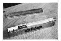
**6)** Place the coiled wire into the coil holder and push up against oblong steel.
