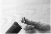
5) Rub Durston lubricant on one side of the wire. This specially formulated Durston lubricant will ensure longer life of the blade and easier cutting.
