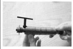
**8)** Place blade holder in Dremel or Foredom flex shaft. Tighten up chuck.
