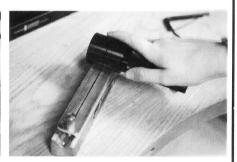
13) Place flex shaft holder over coil holder at the opposite end to the coiled wire. (As picture shows). Start flex shaft holder at slow speed and then gradually work way up to full speed. Then smoothly and slowly move towards you with both hands cutting gently into the wire. When flex shaft holder comes to a stop and has finished cutting, stop the motor and lift of flex shaft holder.
