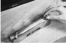
**12)** Screw down holder onto the bench for safety. Place cover over the coiled wire and do up screws firmly but do not over tighten.
