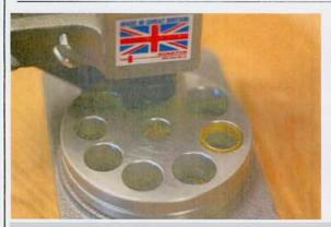
1) Make sure the lever is up right. Place ring in a die which is small than the diameter of the rig. Approximately 20-25% of the ring should stick up above surface.
