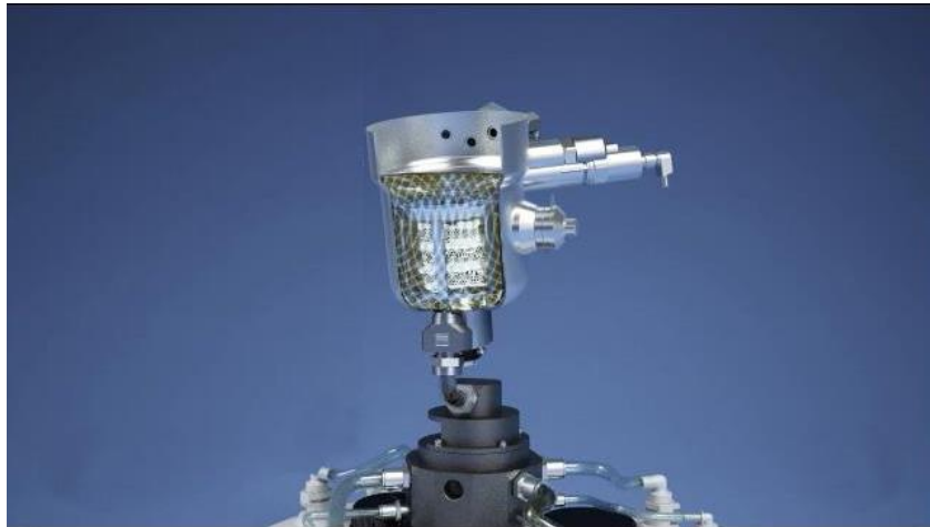
Fig. 3.1.2 View of cleaning basket in cleaning chamber
