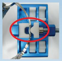
Select the appropriate dies according to the size of the clasp under repair.
