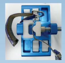
Bend the locking piece as shown to make the clasp tighter. Reverse the direction if too tight!
