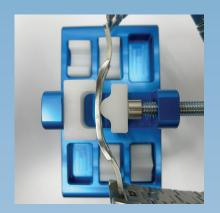
For double locking bracelets, if individual sides lock properly with a good click but difficulty is experienced when locking both sides together (insufficient clearance due to two end pieces touching each other in the center), adjust the middle piece as shown.
