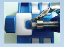
Bend the locking piece as shown to make it tight. Bend only a small amount each time and test the locking until it locks tightly again. Be careful not to overdo it as it is not possible to reverse the bending for this type of clasp.
