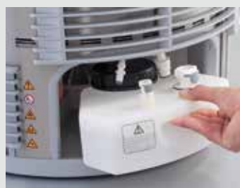
Installing media containers
