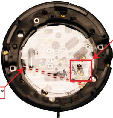
The contact spring must be positioned in the insulator opening
